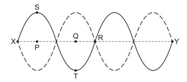
The solid curve shows the string at a position of maximum displacement at time  $t_0$ . The dashed curve shows the other position of maximum displacement. The straight central dashed line shows the mean position of the string.
