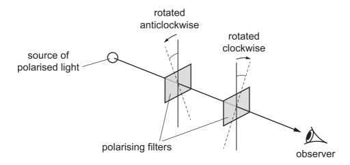
The filters are positioned so that the source appears at its brightest. One of the filters is then rotated clockwise and the other filter is rotated anticlockwise through the same angle.
