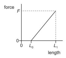
The spring has unstretched length  $L_0$ . When a force F is applied, the spring has length  $L_1$ .
